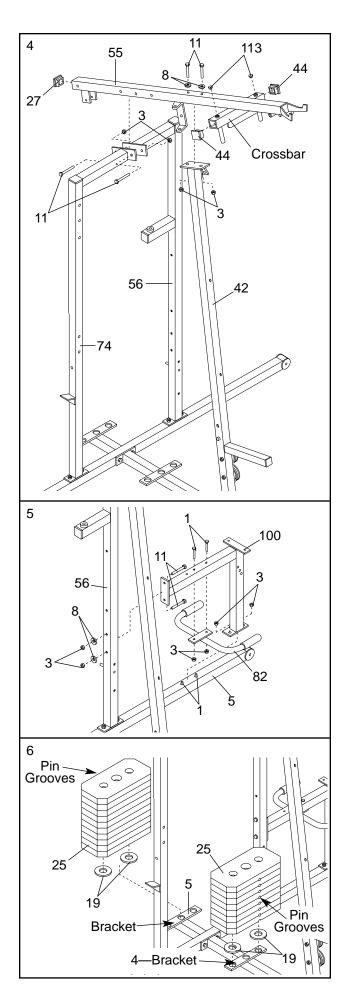
Press a Weight Tube Bumper (64) into the end of the Short Weight Tube (108). Insert the Weight Tube into the front stack of Weights (25). Be sure that the pin on the Weight Tube is sitting in the pin groove in the top Weight.
